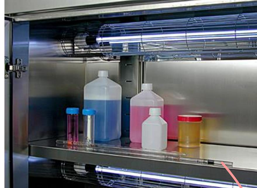
The transparent door with the anti-UV LEXAN® window allow you to check the proper operation at any time.
